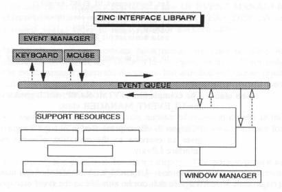
The controlling portion of the UI\_EVENT\_MANAGER class contains a list of input devices that are either polled by the event manager (e.g., a keyboard device) or automatically interrupted by the device's interrupt service routine (e.g., a mouse device).
