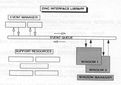
The controlling portion of the UI\_WINDOW\_MANAGER class contains a list of all windows attached to the screen. These windows receive message information from the window manager during an application program. This information is routed to each window according to its position on the screen.
