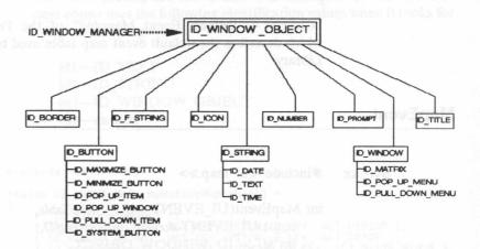
When the MapEvent function is called by a window class object, the closest matching event is returned. For example, the UIW\_TEXT class object matches according to the following event map hierarchy:
